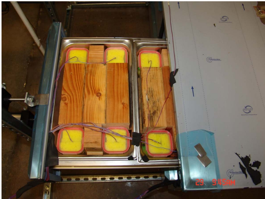
FIGURE 4. PHOTOGRAPH OF OPEN CHEF BASE DRAWER WITH FILLER PRODUCT AND SIMULATED FOOD PRODUCT
