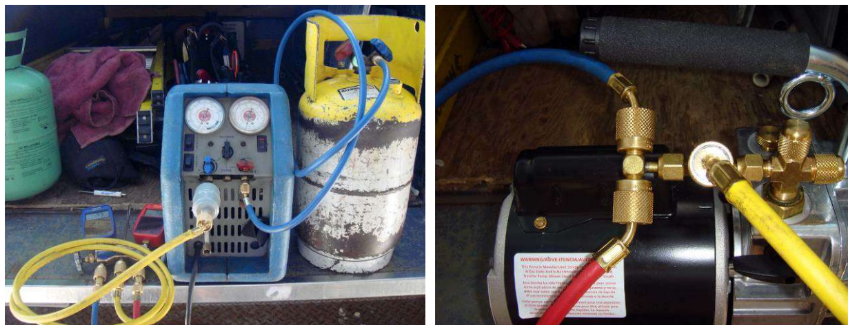
Figure 4.1 Purging Refrigerant from Manifold Using Recovery Tank and Vacuum Pump
