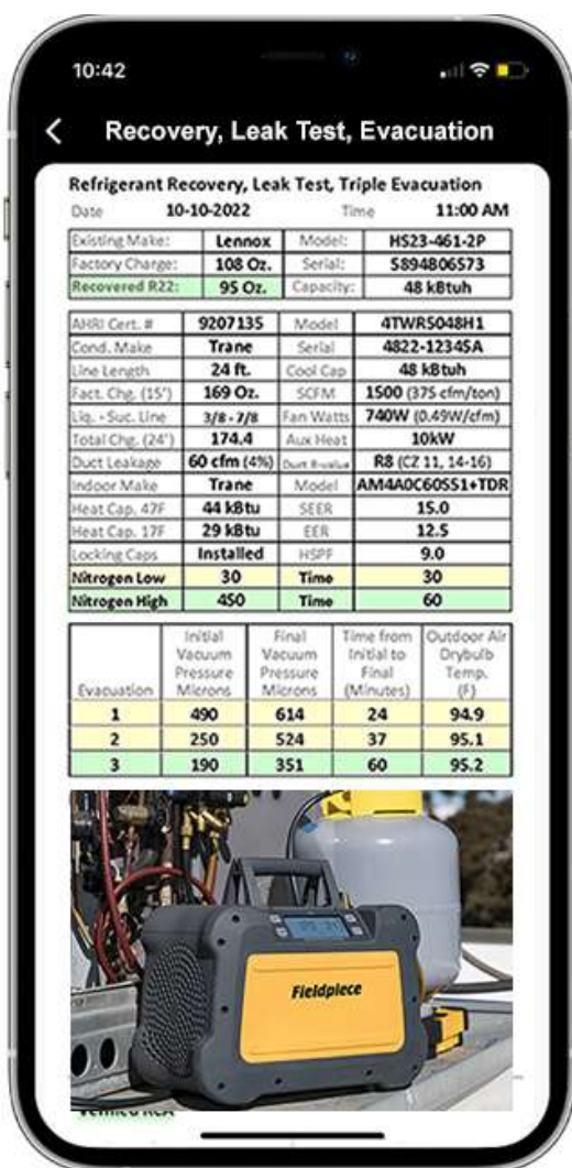
Figure 3.17 Recovery, Leak Tests, and Triple Evacuation
